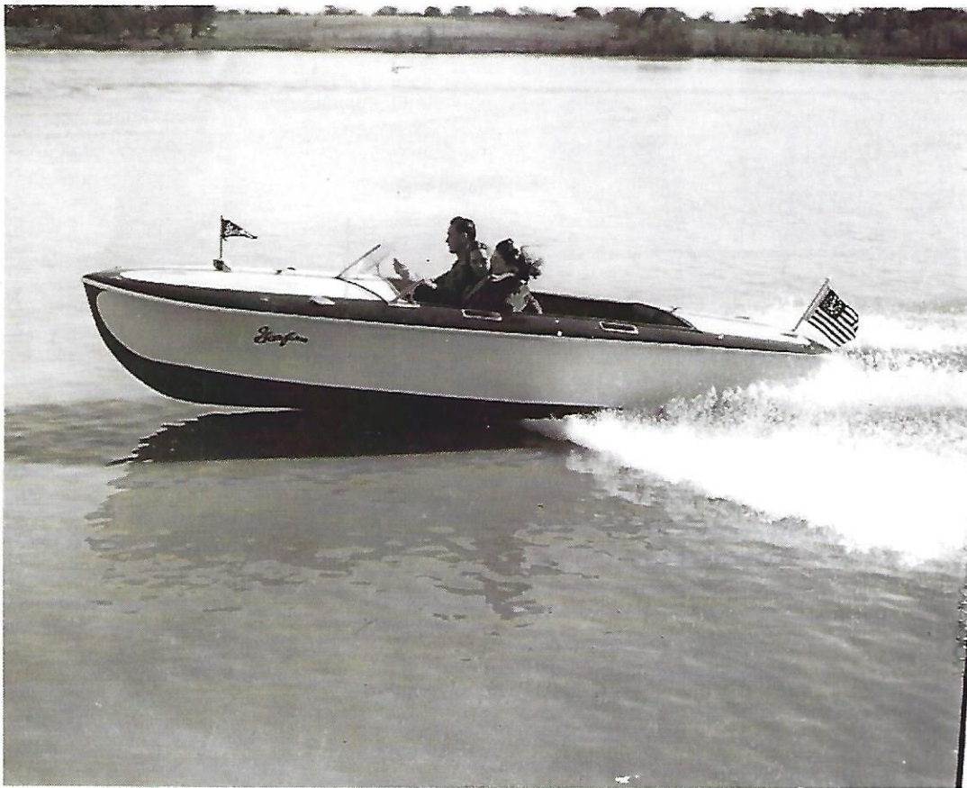
A good view of the 16'-8" Garform Sportabout powered with the optional Gray Phantom Four-45 HP engine that provides speeds to 34 mph.
