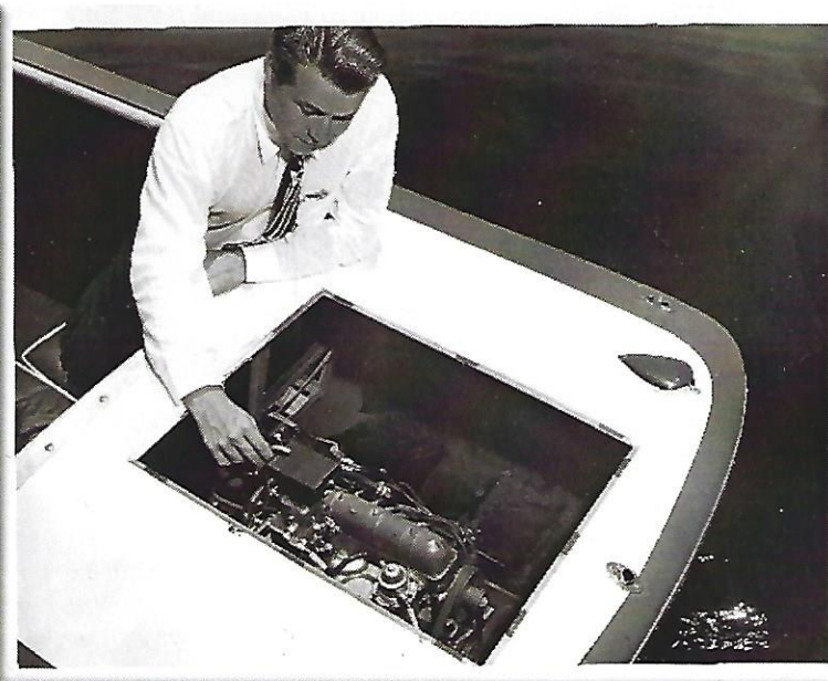
Gar Wood, Jr. inspects the installation of the 26.5 HP Crosley Cobra engine in his 16-foot Garform runabout. The 4-cylinder engine weighs just 59 pounds and will turn 5400 r.p.m.'s at full throttle.
